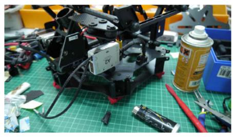
Degrease the MCU support and the MCU itself, and apply 3M PE Foam or 3M VHB. Degreasing is essential (use Isopropyl alcohol from 3M, it's a very good product). You can protect the antennas of the A2 integrated receiver with nylon braid, but make sure that the braid does not « pull » the antennas from the MCU once nylon braid are installed and tensionned.
