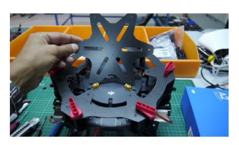
Remove the top frame « star » carbon part and then the powerboard plastic cover. Take care by the way to check all screws on the frame and re apply medium strenght threadlock.
