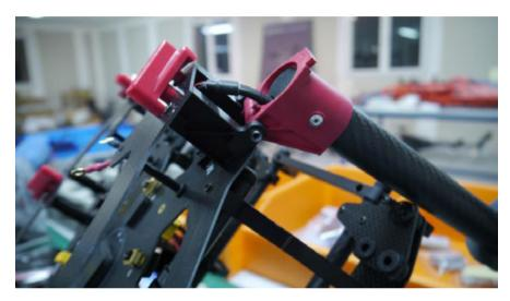
Install the booms and att thread lock in the boom supports as the nylon lock installed in factory will wear out very quickly. Tighten the screws so that the arms cannot « fall » by themselve when unlocked. Remove the heatschrink from the crimped connector and secure with soldering. Put back a heatschrink sleeve.
