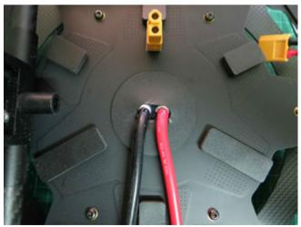
Remove one (left or right) landing gear retract unit So you can remove the carbon tube. You can apply Plastidip on the solderings of the main power cables. Some poeple put also nylon braid on these cables but It is not really necessary. But you can add 2 thickness Of small heatschrink lenght on the cables where they Are clamped on the frame with the small alu parts.
